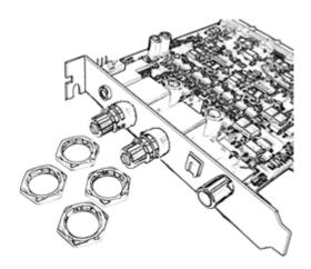
5. Insert the Overture 192 card into the PCI slot carefully and push the card firmly until it is seated securely, then screw the Overture 192 bracket to the chassis of your computer.
